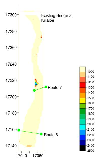
Figure I.8: 2-Dimensional Contour Plot of Magnetic Deviation Acquired from the Site Survey. Data Range from -1000 nT to -2500 Nt on a Background of -1000 nT
