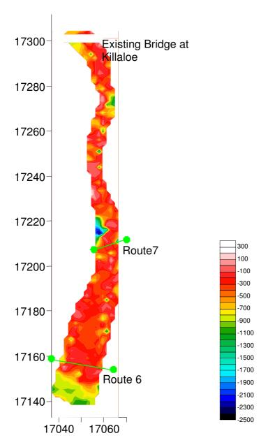
Figure I.7: 2-Dimensional Contour Plot of Magnetic Deviation Acquired from the Site Survey. Data Range from +300 nT to -2500 Nt on a Background of -200 nT
