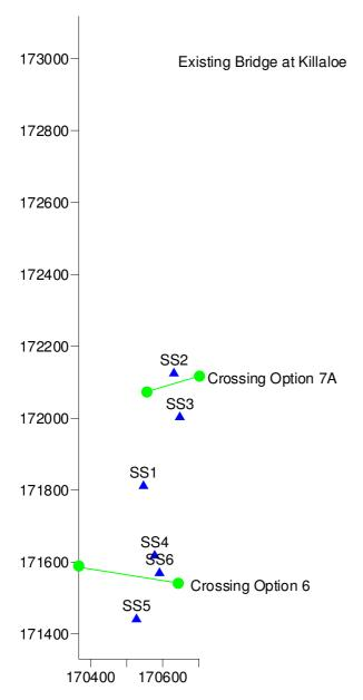
Figure I.19: Location of the Anomalies Interpreted from the Sidescan Record in Relation to the Proposed Crossings (Scale to Irish National Grid)
