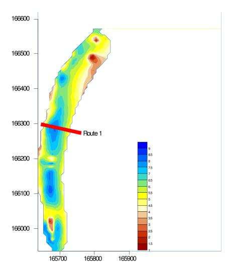
Figure I.6: 2-Dimensional Contour Plot of Bathymetric Data Obtained over the Study Area at O'Briensbridge/Montpelier
