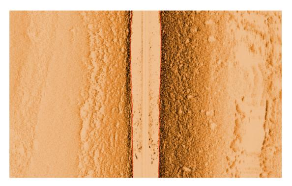
Figure I.3: Sonar Image Displaying the Hard Rock/Gravel Riverbed Within the Study Area.
