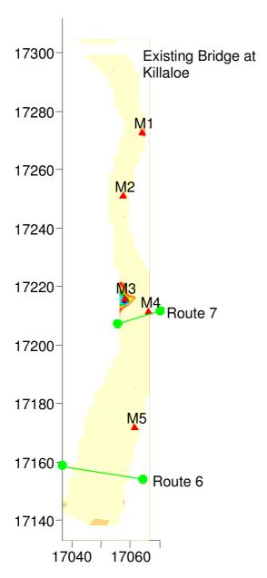
Figure I.9: The Location of Magnetic Anomalies M1-M5
