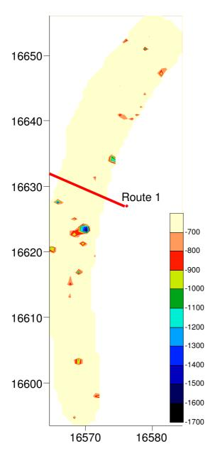
Figure I.11: 2-Dimensional Contour Plot of Magnetic Deviation Acquired from the Site Survey. Data Range from -700 nT to -1700 Nt on a Background of -600 nT
