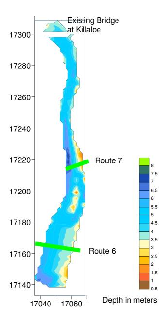
Figure I.4: 2-Dimensional Contour Plot of Bathymetric Data Obtained over the Study Area at Killaloe/Ballina
