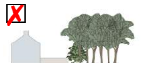
Trees too close to back gardens - shading, falling branches
