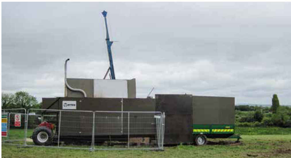
A modern drill rig, enclosed to reduce noise, operated by Lundin Mining in the mineral exploration at Kilbreckan.
