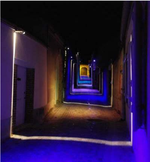
Bow-way lighting: varying combinations of LED coloured Flood Optic (I-Pro) and Blade Effect Optic (Trick RGB), wall or ceiling mounted, as supplied by iGuzzini or similar
