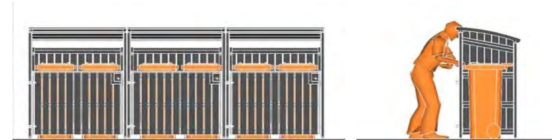
Communal bin storage (MetroStor or similar) 770L-1280L 4-wheel bins 1330mm(D) x 3100mm(W) x 1816mm(H)
