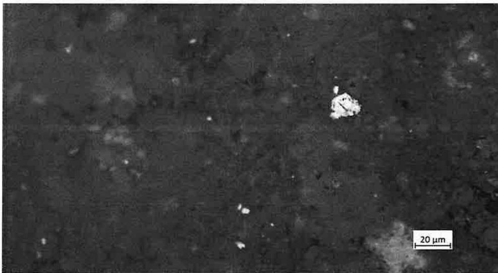
Unoxidised microcrystalline pyrite in matrix. [Scale 20 µm, Reflected light]
