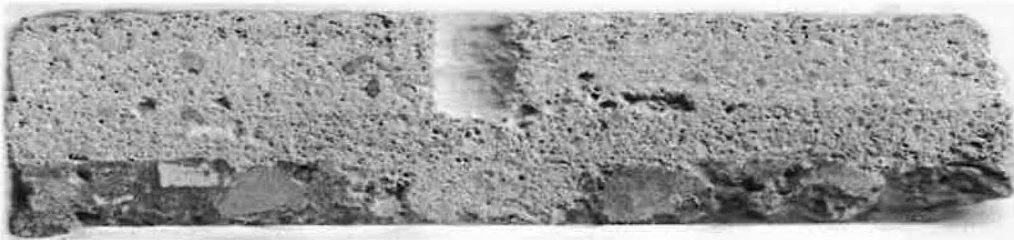
Two coat render of similar composition. Outer coat is 8mm thickness, inner coat is 5mm.
