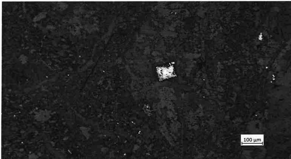
Unoxidised crystalline pyrite in a packstone [Scale 50 µm, Reflected light]
