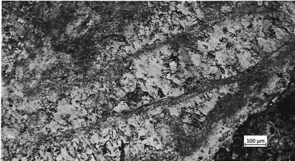
Recrystallised limestone. [Scale 100 µm, Cross polarised light]
