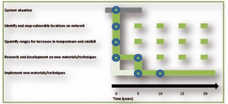
Figure 4.2 Pathways map of options to increase resilience of wet-mix macadam and surface dressed roads to increased temperature and precipitation.
