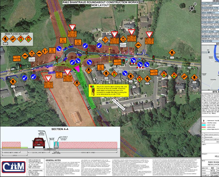
DESIGN PARAMETERS CHAPTER 8 ROAD LEVEL: SPEED LIMIT: 60km/h ROADWORKS TYPE NUMBER OF SIGNS SIGN VISIBILITY: 60m DISTANCE BETWEEN SIGNS: 20m SIGNS SIZE RECTANGULAR - MIN. 600mm SIGNS SIZE CIRCULAR - MIN. 600mm CONE HEIGHT - MIN.: 750mm FAPER CONE SPACING LONGITUDINAL CONE SPACING: RATE OF TAPER: LANE - 45°; HS - 1 IN 10m SAFETY ZONE: LONGITUDINAL - 15m; LATERAL 0.5m CUMULATIVE AWS DISTANCE: MAXIMUM LENGTH OF SHUTTLE MINIMUM LANE WIDTH:
