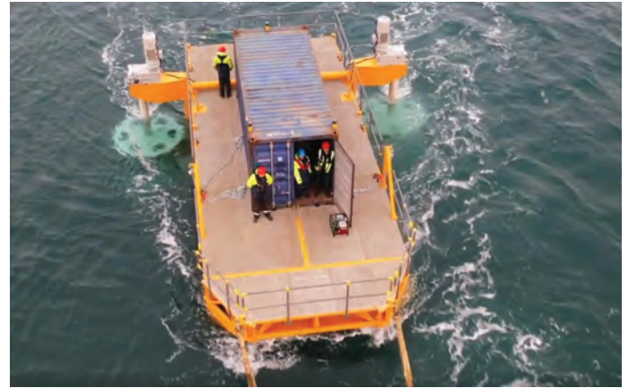
60Kw tidal test device to be deployed off Cahercon Pier.
